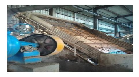
2. Application of inclined screens instead of traditionally used rotating thickeners and disc filters for thickening the mass. Simplifies construction and reduces energy costs. Inclined screens have no drives and any rotating elements.
